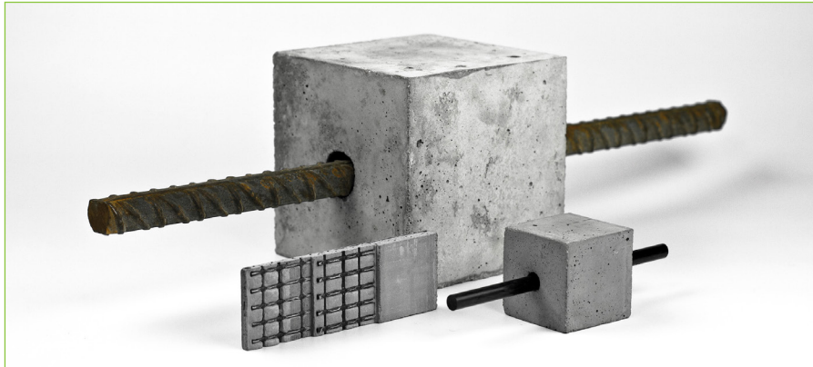
Demonstrator, comparison of a steel rod, a carbon composite rod and textile-reinforced concrete (© filmaton)
