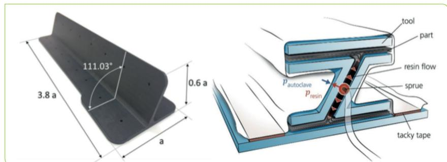
Fig. 1: Composite stiffener dimensions (left) and the aluminium tool concept used (right)
