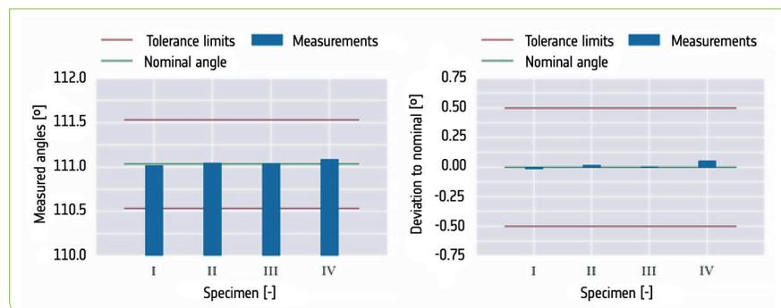
Fig. 4: Cross-section evaluation of the four manufactured composite profiles
