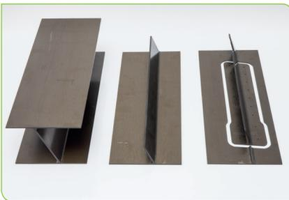
Fig. 2: Manufactured CFRP component, segmented frame and final component developed by Embraer, Toho Tenax and DLR
