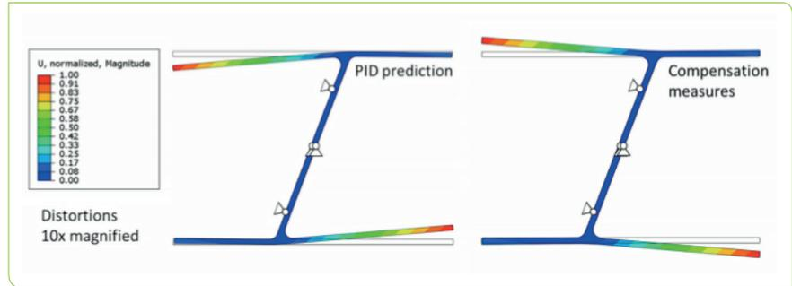
Fig. 3: Normalized PID predictions and compensation measures derived through the P-approach
